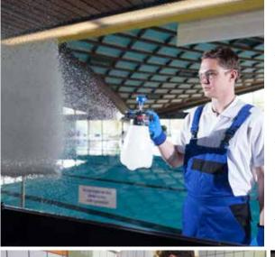
The use of foam for cleaning purposes is gaining popularity. Advantages are visibility and longer chemical effect with no run-off. In many cases foam is used for surfaces that require a reduced moisture level.
